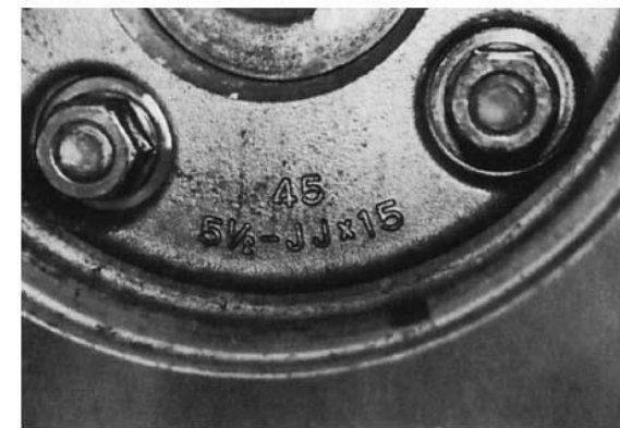
FIGURE 20-28 The size of the wheel is usually cast or stamped into the wheel. This wheel is 5 1/2 in. wide. The letters JJ refer to the contours of the seat area of the wheel.
