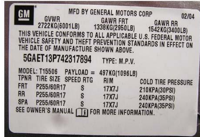
FIGURE 20-13 A typical door placard used on a General Motors vehicle indicating the recommended tire inflation. Note that the information also includes the tire size and speed rating of the tire as well as the recommended wheel size.
